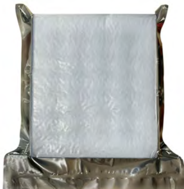
Seal the Tray with Anti-Static Bag
